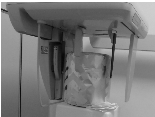
Fig. 1 – The picture shows a skull stabilized in the cephalostat on an aluminum filter cylinder.
